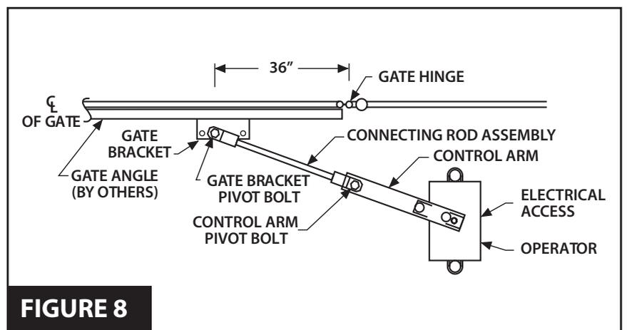
**Note: Adjustment can be made in (4) locations to get desired closed position, as described below. Always start with Option "a".**
