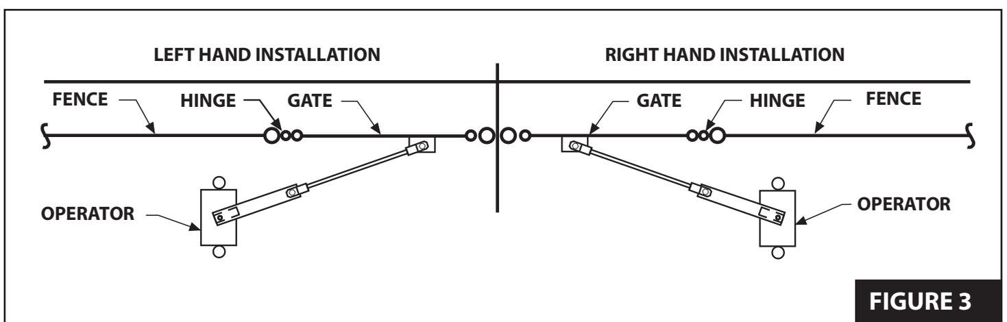
1. Gate must swing freely to fully opened and fully closed position.
