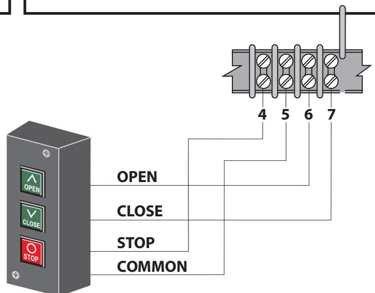
1. Connect a wire from the **COMMON** connection of the control station to Terminal #5.
