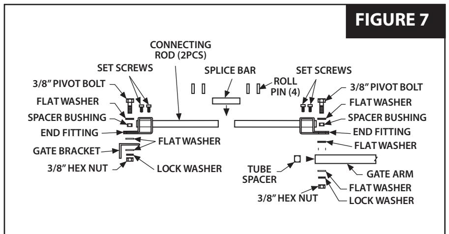
4. Install gate bracket on remaining end of connecting rod (See **Figures 7 & 8**)
