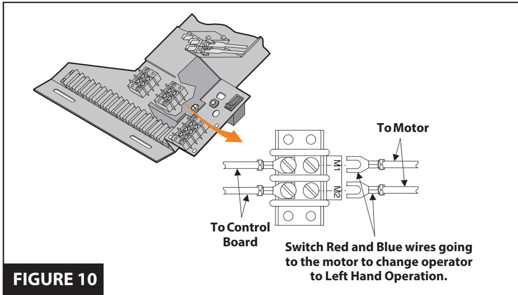
To convert operator to left hand operation, make certain the power switch is **OFF**, and locate the motor terminal strip (See **Figure 10**). Switch the red and blue wires, between M1 and M2, that go to the motor. The operator is now setup for left hand installation.
