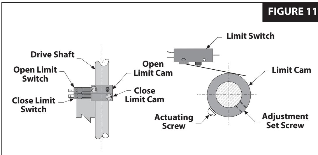
1. Turn on power. Press **OPEN** button on control station. Gate should stop before full open position is reached. If gate does not stop when open position is reached, **PRESS STOP BUTTON!**
