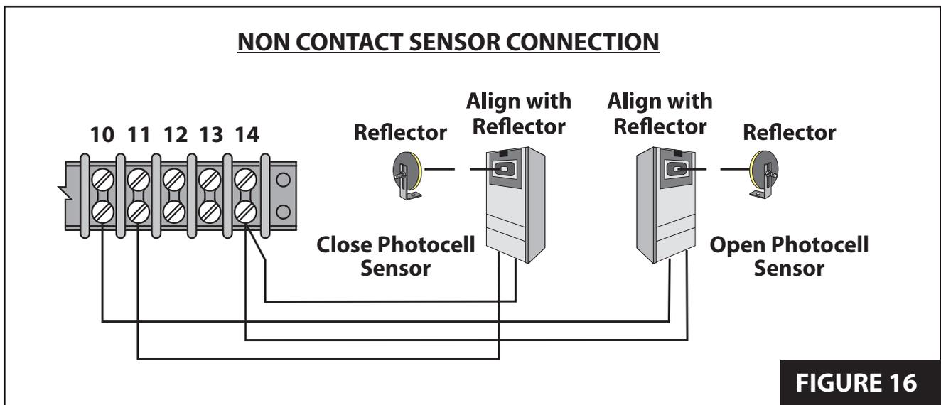
**NOTE:** Close photocell is connected to **Terminal #11** and **Terminal #14**. Open photocell is connected to **Terminal #10** and **Terminal #14**.
