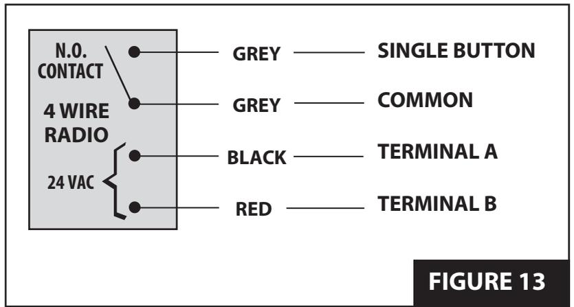
**NOTE:** If your radio's connecting wires are not color coded as shown, see the radio's installation manual to determine which wires are for the normally open contacts and which require the 24VAC Power Supply.
