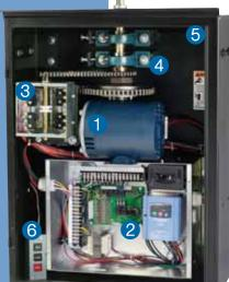
ODirect C-Face Motor to Gear Box Drive
