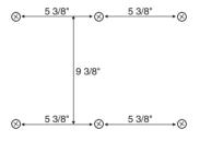
MOUNT CABINET WITH SUITABLE HARDWARE FOR MOUNTING SURFACE.
