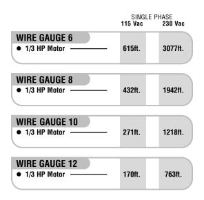
**NOTE:** Calculated using NEC guidelines. Local codes and conditions must be reviewed for suitability of wire installation. All power wiring should be dedicated and protected. Location of primary power disconnect should be labeled.
