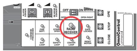
**Symptom:** The radio receiver LED on the control board remains **“OFF”** when using the remote control.
