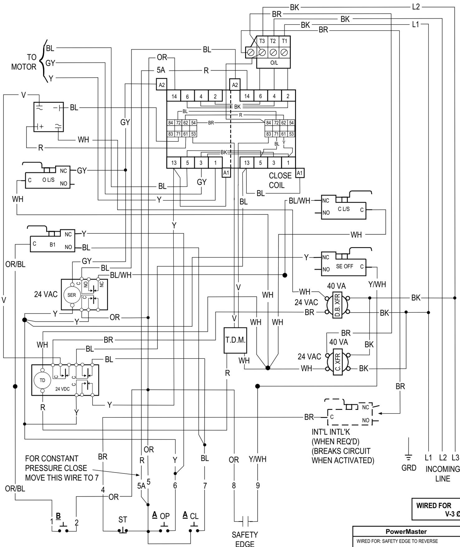
**A** TREADLES, PULL SWITCHES, KEY SWITCHES, WANDS, PHOTOELECTRIC DEVICES, ETC. MAY BE CONNECTED WHERE INDICATED.
