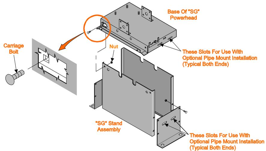
2. Using 1/2" hardware (Not Supplied) bolt assembled unit to the pad, being sure to align operator parallel to the fence.
