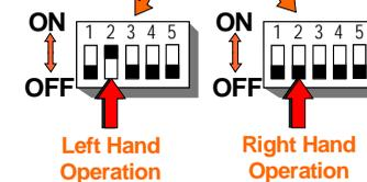
**NOTE:** This unit is factory setup for **RIGHT HAND** operation. To convert operator to left hand operation move dipswitch #2 to on position.
