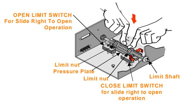
16. After the desired open and close position of the gate has been obtained, make certain that a groove in both limit nuts are engaged by the pressure plate.
