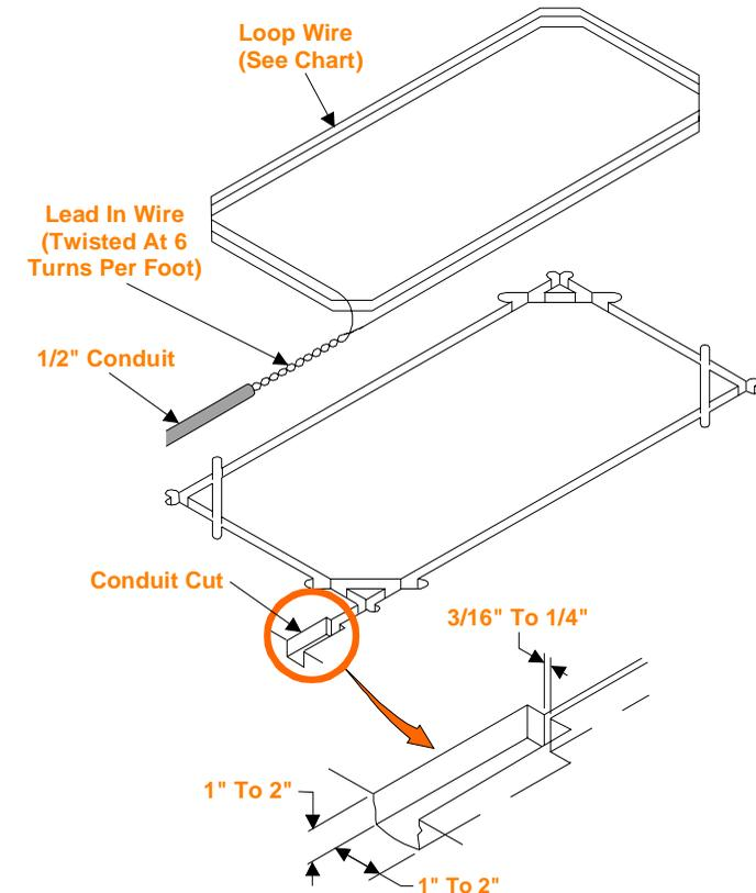
3. Leaving enough wire for the **LEAD IN**, insert the specified number of turns of wire in the cut grooves. (See chart).
