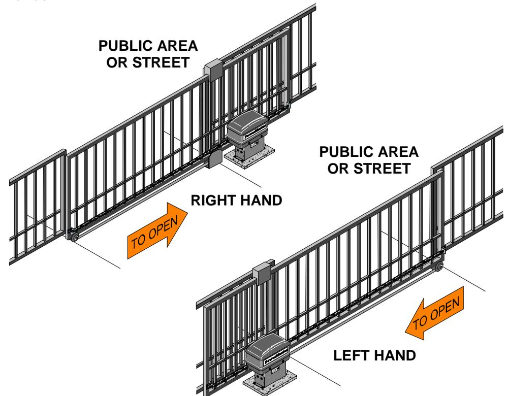
1. Gate must slide freely to fully opened and fully closed position.
