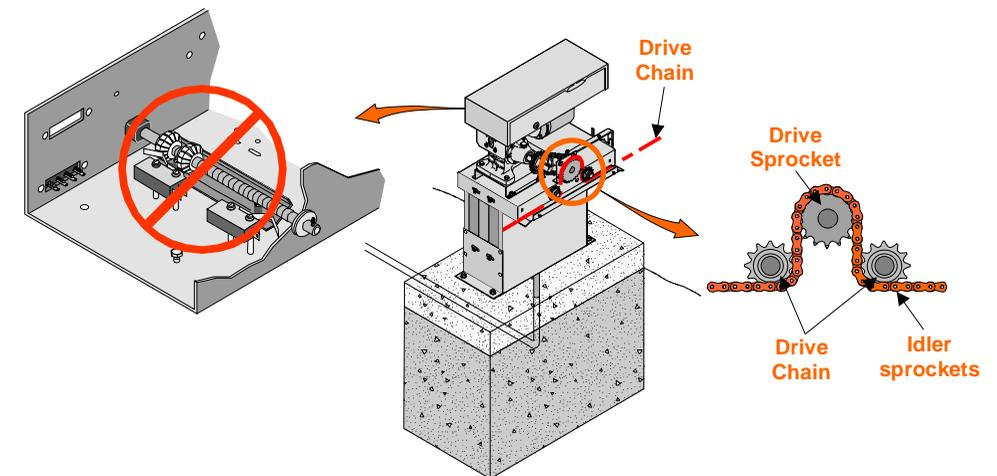
7. Pull the chain through to the opposite end of the gate. Cut the chain to the correct length, attach remaining chain take-up bolt and install in the gate bracket as in steps 2 through 4.
