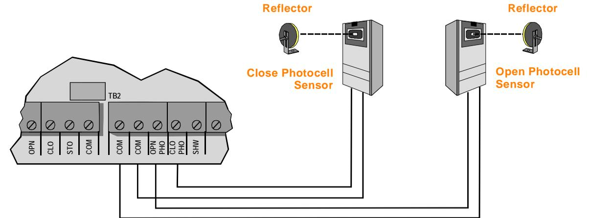
**NOTE:** Close photocell is connected to “**CLO PHO**” and “**COM**” terminals. Open photocell is connected to “**OPN PHO**” and “**COM**” terminals.
