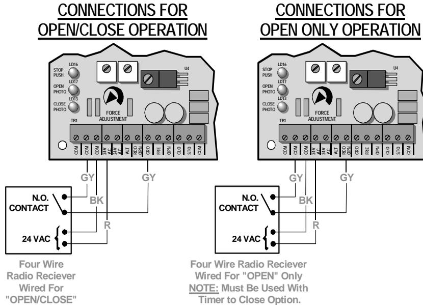
1. For electrical connections of a four-wire radio receiver via the external terminal strip. See below.
