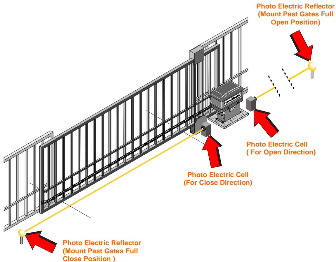
3. Connect **NON-CONTACT** sensors to the control board as shown below.
