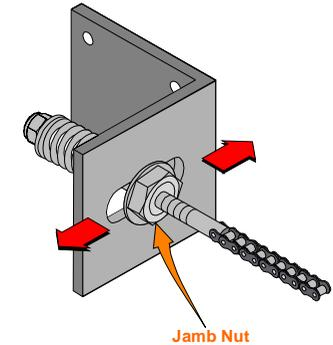
11. Adjust chain tension so that the chain tension springs are reduced to a length within 1-7/8" and 1-3/4".
