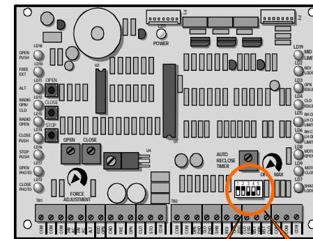
Place Dipswitch #2 In "ON" Position For Left Hand Operation And "OFF" Position For Right Hand Operation.
