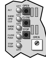
**NOTE:** If Dipswitch #3 is in the "ON" position for use with a **NORMALLY CLOSED "STOP" BUTTON**, then the board mounted "STOP" button must be held depressed in order to use the open and close buttons. Releasing the stop button will then stop the operator.
