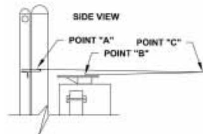
These measurements will be needed when placing an order for special length crank extensions and links. Also note that the measurements you have just calculated are center to center only, and are not overall dimensions, which would also include other attachment hardware, such as gate arm clamps.
