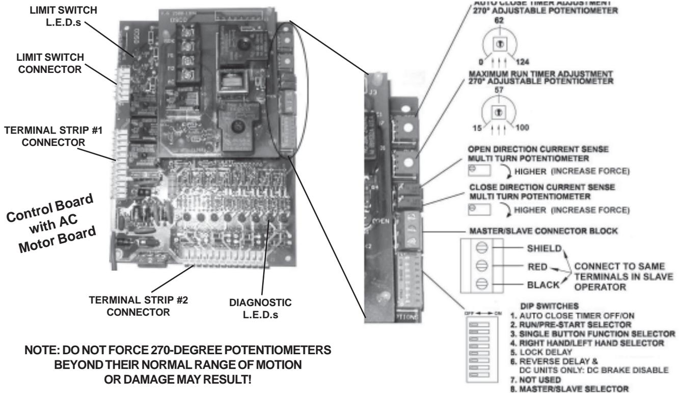
**NOTE: DO NOT FORCE 270-DEGREE POTENTIOMETERS BEYOND THEIR NORMAL RANGE OF MOTION OR DAMAGE MAY RESULT!**
