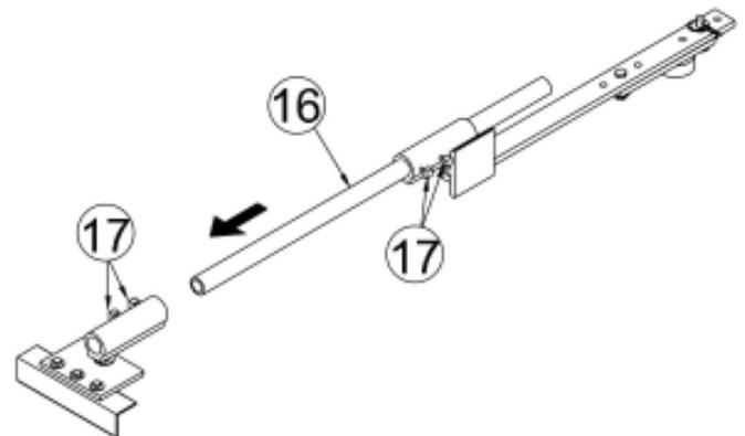
Slide the pipe link (16) through the arm assembly as shown. Place the 5/16" square bolts in the gate clamps (17) and tighten carefully. **Do not overtighten!**
