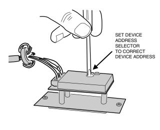
SET DEVICE ADDRESS SELECTOR TO POSITION 1-6 (MUST BE SET DIFFERENT FROM ANY OTHER REMOTE DEVICE IN THE SYSTEM)
