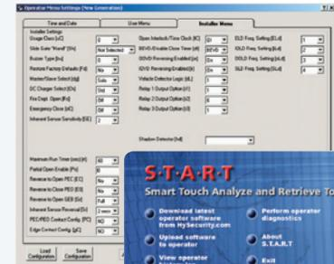
Smart Touch Analyze and Retrieve Tool allows users to upload latest operator software, download fault logs, generate diagnostics, and program the operator using a laptop.
