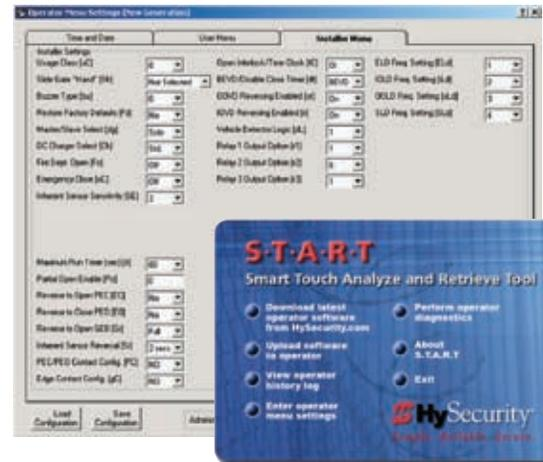
Smart Touch Analyze and Retrieve Tool allows users to upload new operator software, download fault logs, generate diagnostics, and program the operator.
