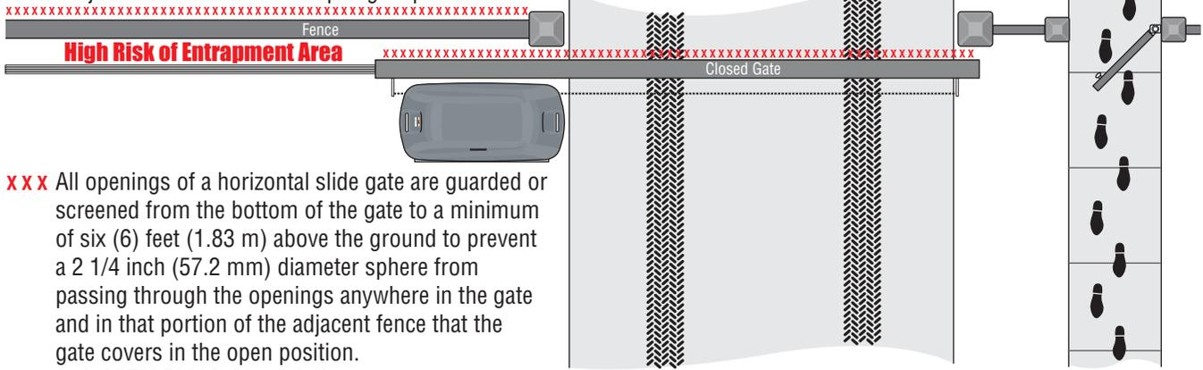
**xxx** All openings of a horizontal slide gate are guarded or screened from the bottom of the gate to a minimum of six (6) feet (1.83 m) above the ground to prevent a 2 1/4 inch (57.2 mm) diameter sphere from passing through the openings anywhere in the gate and in that portion of the adjacent fence that the gate covers in the open position. (ref. ASTM F2200-11a, 6.1.2)
