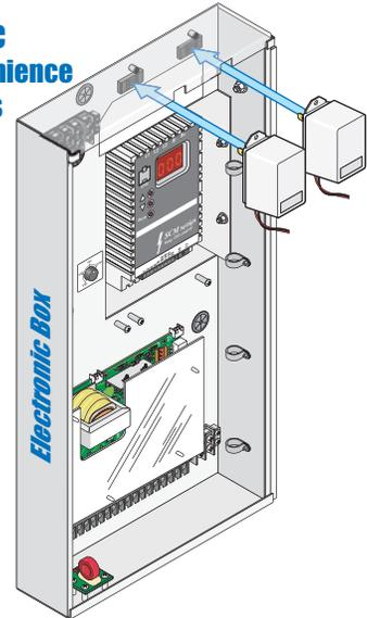
**1 OPEN Entrapment Sensor (Photo Sensor):** Obstructed opening-direction photo beam will stop the gate **during the opening-direction only**. Gate will resume the open cycle when the obstructed photo beam has been cleared.
