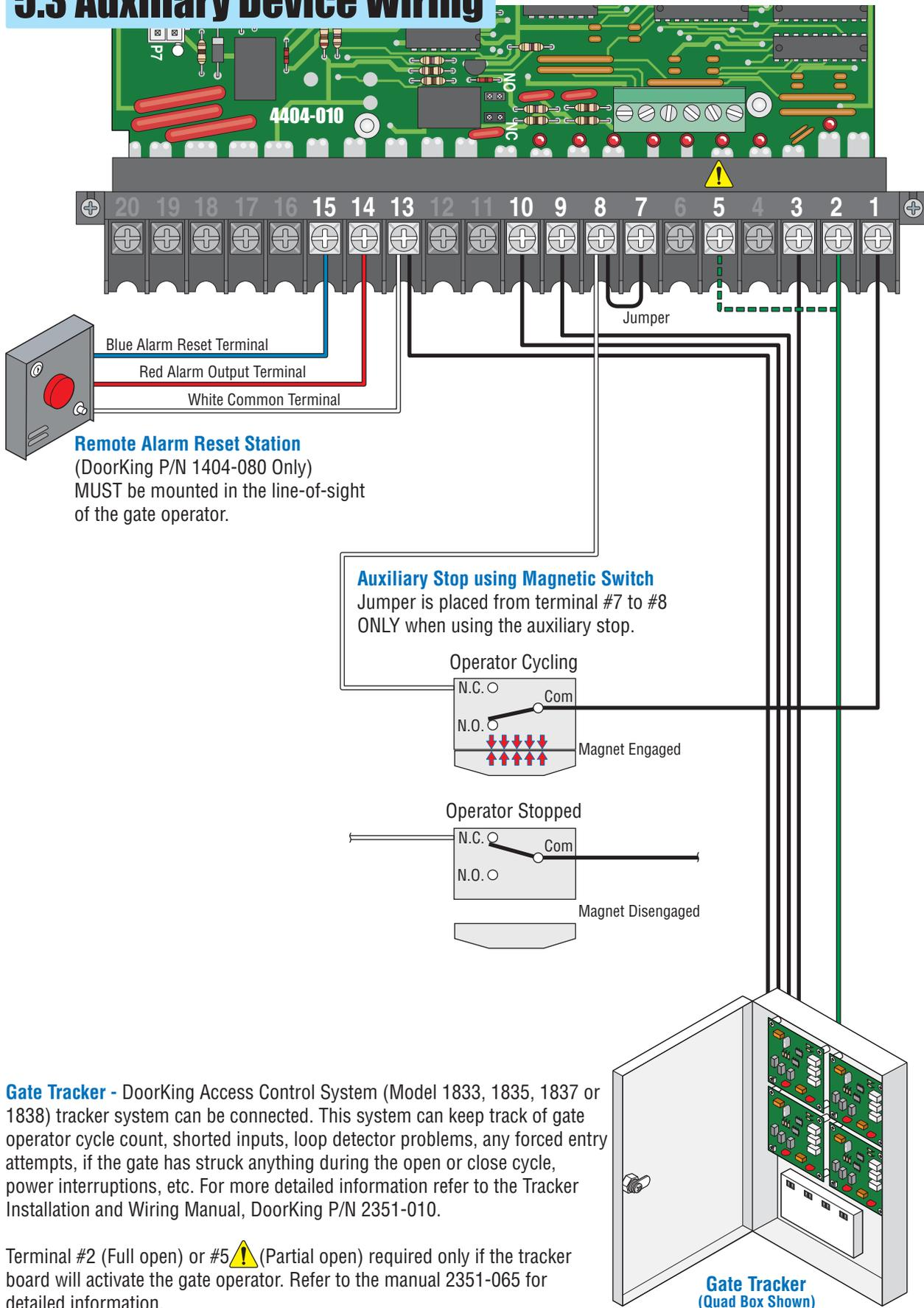
**Gate Tracker** - DoorKing Access Control System (Model 1833, 1835, 1837 or 1838) tracker system can be connected. This system can keep track of gate operator cycle count, shorted inputs, loop detector problems, any forced entry attempts, if the gate has struck anything during the open or close cycle, power interruptions, etc. For more detailed information refer to the Tracker Installation and Wiring Manual, DoorKing P/N 2351-010.
