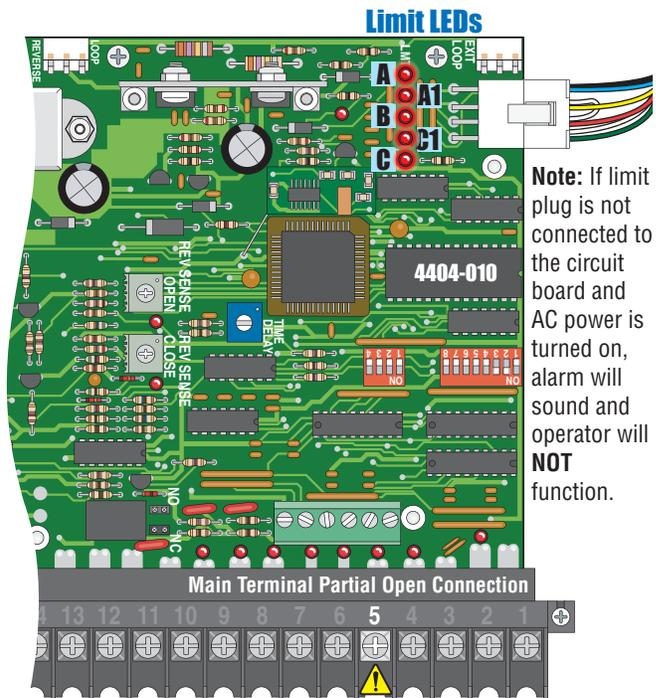
**Note:** If limit plug is not connected to the circuit board and AC power is turned on, alarm will sound and operator will **NOT** function.
