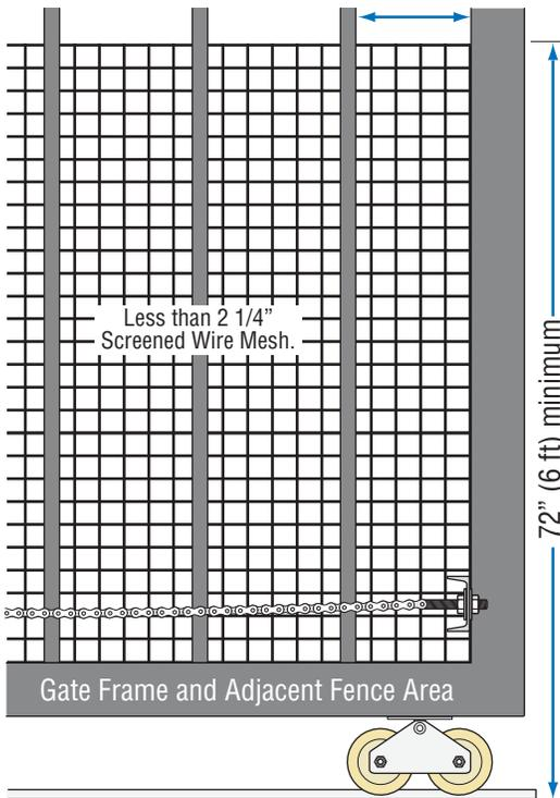
Note: Install screened wire mesh to an existing non-compliant gate and the adjacent fence that covers open gate position (See above).
