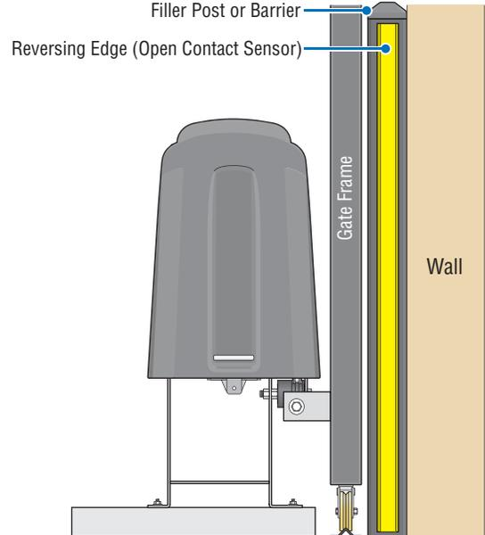
A filler post or barrier may need to be installed between the gate and wall area to reduce the distance to 2 1/4" or less. A reversing edge should be installed on the post or barrier for safety (See page 8 for more information).
