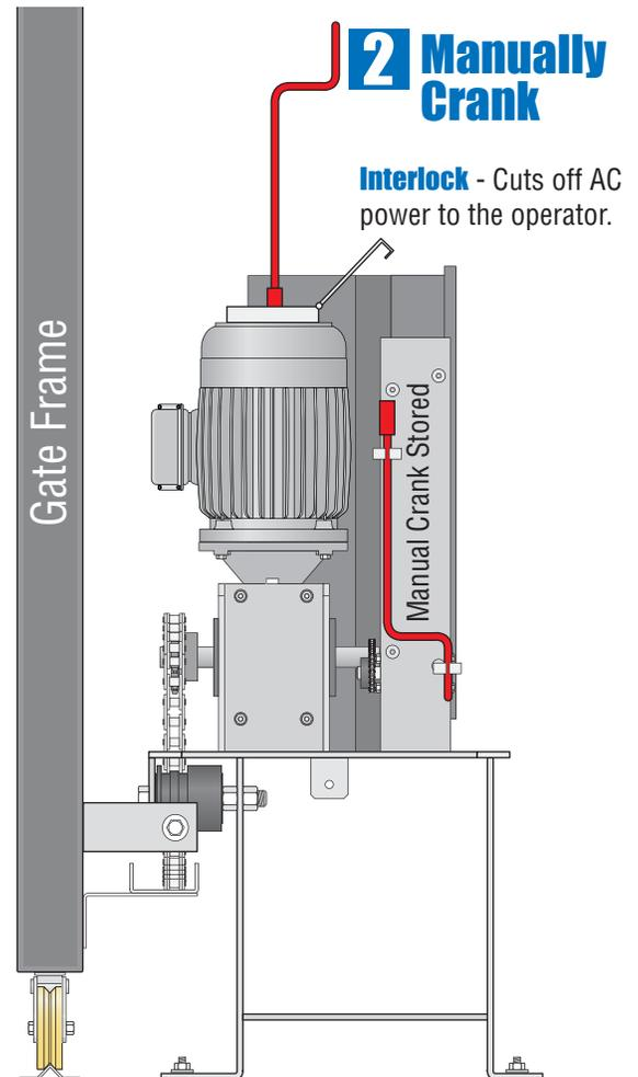
Insert the supplied manual hand crank into the motor shaft underneath the interlock door. Turn the crank to open the gate. Mechanical disc brake on 9555 operator **MUST** also be manually released before manually turning the hand crank.
