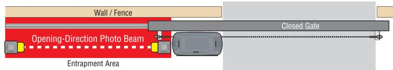
**2 CLOSE Entrapment Sensor (Photo Sensor):** Obstructed closing-direction photo beam will stop the gate **during the closing-direction only**. Gate will resume the close cycle when the obstructed photo beam has been cleared.
