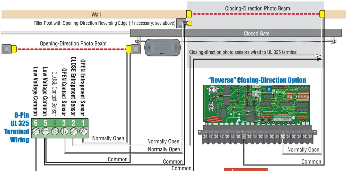
IF the closing-direction photo sensor is wired to the UL 325 terminal, a closing-direction photo beam that gets obstructed will **STOP** the gate, then resume closing the gate when the obstructed photo beam has been cleared.
