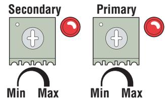
The ideal adjustment will allow the operator to move the gate through its entire travel cycle without reversing, but will reverse upon contact with an obstruction with no more than 40 Lbs of force. This force can be measured with a gate scale, DoorKing P/N 2600-225.
