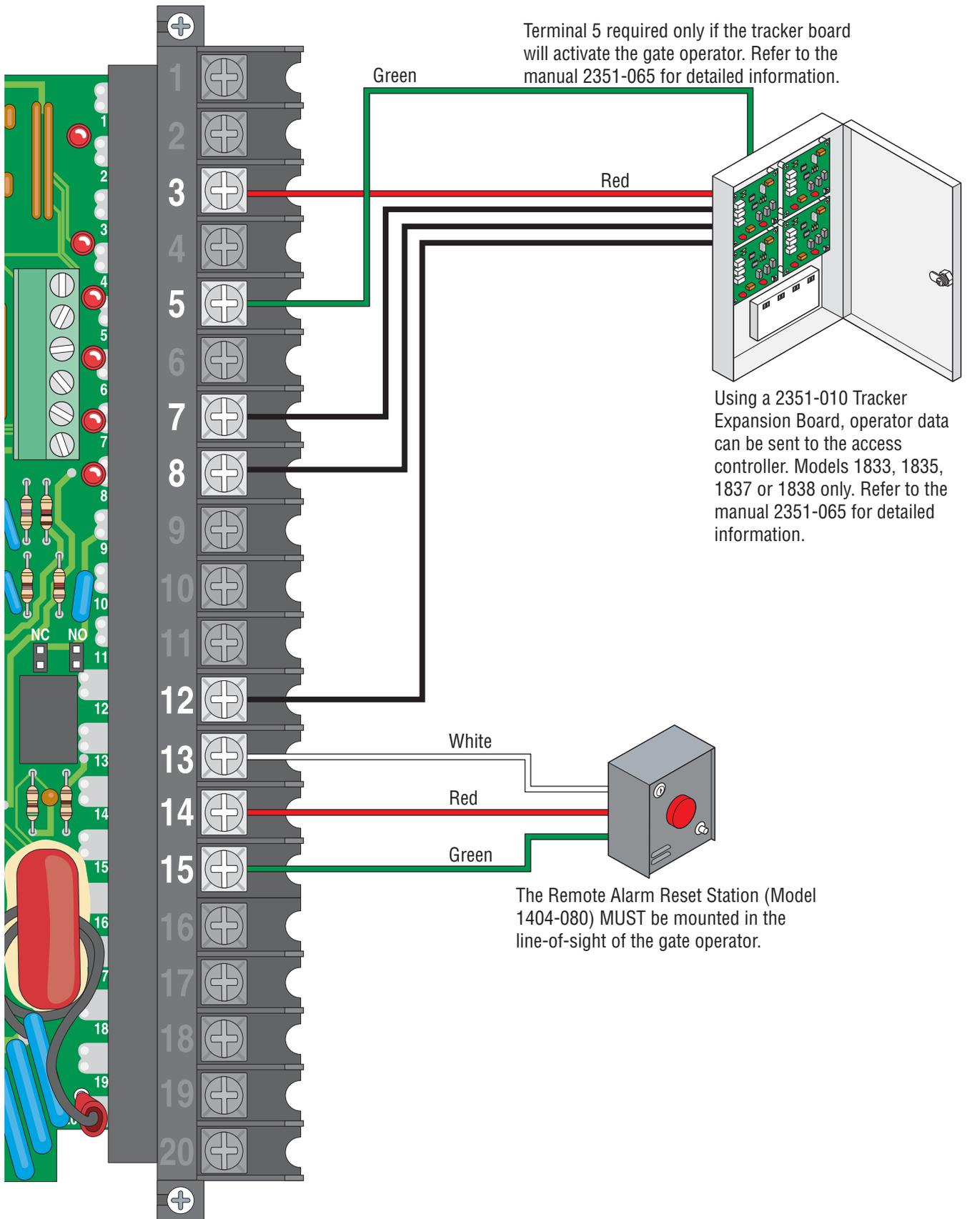
Terminal 5 required only if the tracker board will activate the gate operator. Refer to the manual 2351-065 for detailed information.
