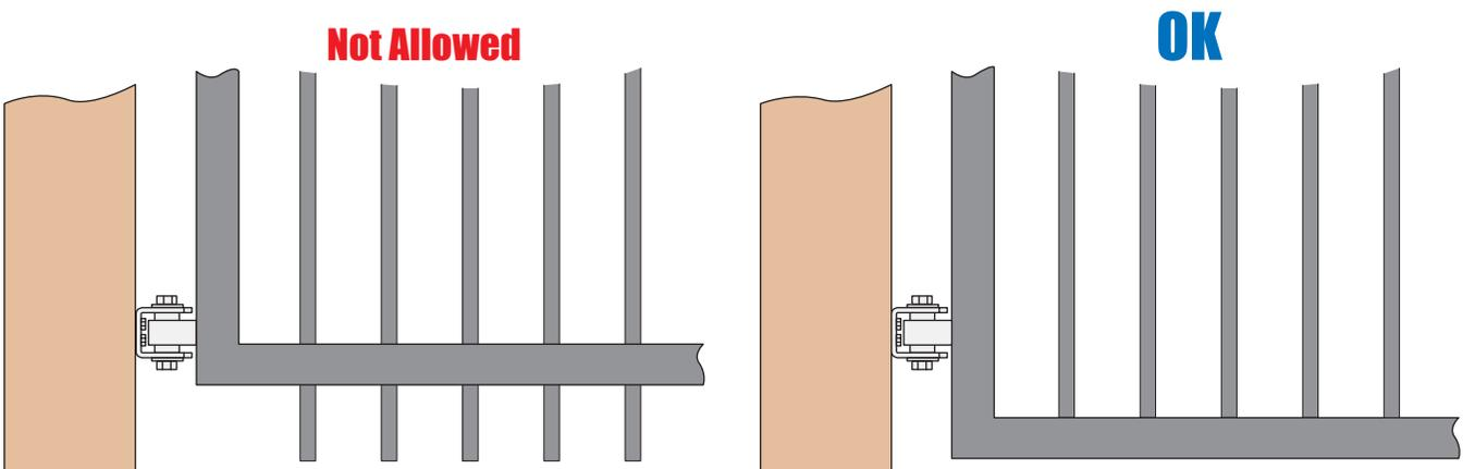
Gates shall have smooth bottom edges, with vertical bottom edged protrusions not exceeding 0.50 inches. ASTM F2200 4.3
