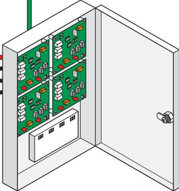
Using a 2351-010 Tracker Expansion Board, operator data can be sent to the access controller. Models 1833, 1835, 1837 or 1838 only. Refer to the manual 2351-065 for detailed information.
