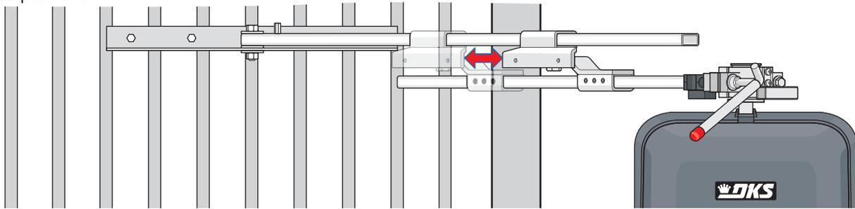
Mark and cut off excess arms. Secure arms to elbow assembly with 6 allen screws. Tighten hub and replace release tool. Install safety covers.
