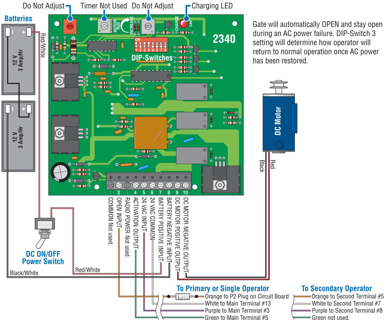
Gate will automatically OPEN and stay open during an AC power failure. DIP-Switch 3 setting will determine how operator will return to normal operation once AC power has been restored.
