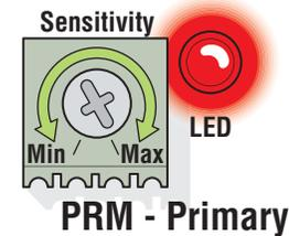
**Safety Note:** The LED will remain ON after a cycling gate gets obstructed during **normal** operation to indicate that the reverse sensor has been tripped. Always check the gate area for possible obstructions before putting operator back in service.
