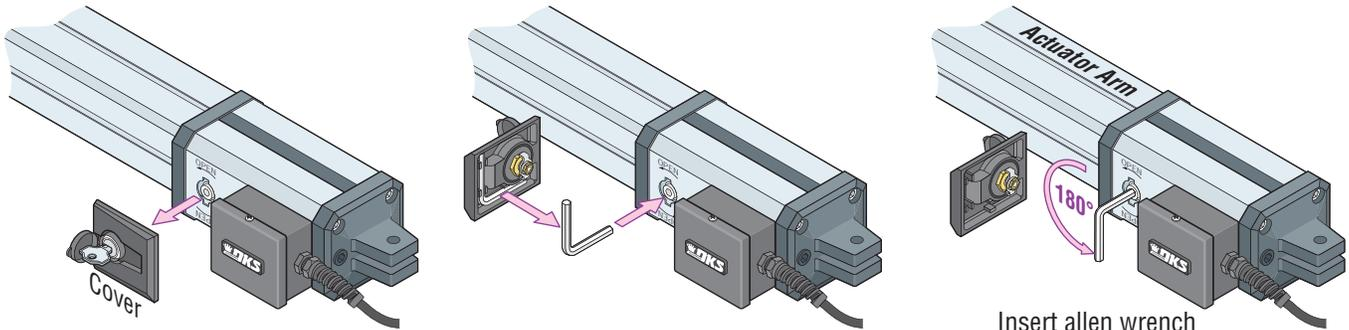
Use key to unlock and remove the cover. Remove allen wrench from inside of cover.
