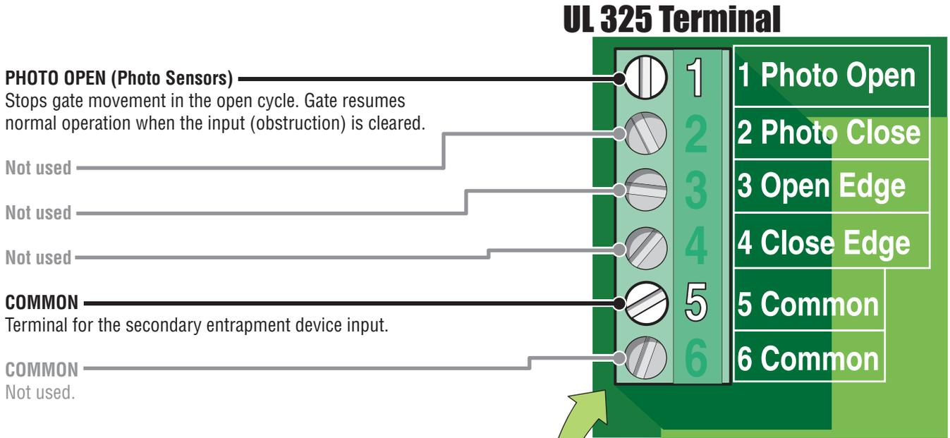
**UL 325 Terminal Note:** The 6-pin terminal can be unplugged from circuit board for easy wire connections.
