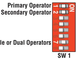
**Note:** 3 and 5 limit LEDs can be **Open** or **Close** limits depending on SW 1, switch 1 and 2 settings (See page 17).
