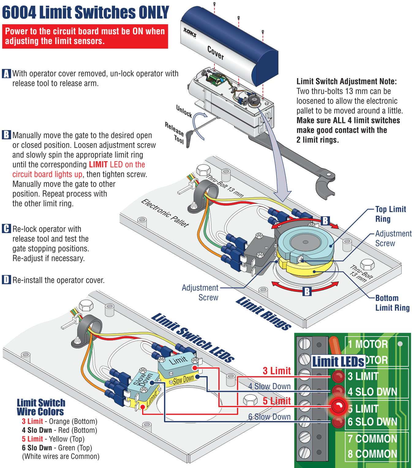
**E** Adjust the Secondary operator limit rings if dual operators have been installed. SW 1, switch 2 controls secondary operator opening direction. SW 1, switch 7 **MUST** be ON when using dual operators (See page 18).
