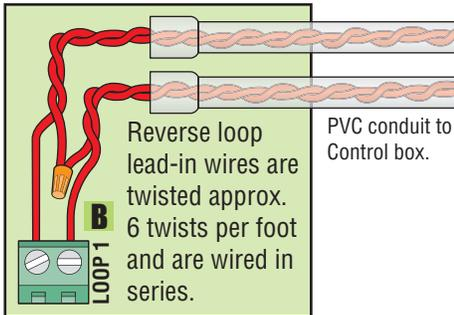
Loop detector wiring is shown for DoorKing plug-in loop detectors P/N 9409-010 and P/N 9410-010 only. If other loop detectors are used, refer to the installation instructions supplied with those detectors for wiring and separate power instructions.
