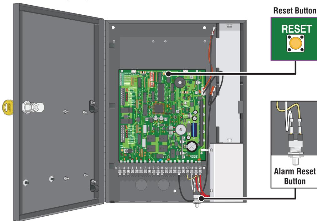
Once the gate has been reset, an open or close command is needed to start the gate operator. Most activating commands will cause the gate operator to cycle to the open position. This includes activation of a key switch or open command and activation of the automatic exit loop (If used). Activation of a close command will run the gate to the closed position.
