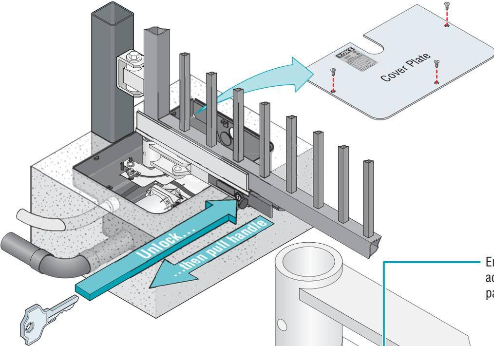
**B** Manually move the gate to the desired open or closed position. Loosen limit nut and slowly slide the limit assembly until the corresponding **LIMIT LED on the circuit board lights up** and tighten nut. Manually move the gate to other position. Repeat process with the other limit assembly.
