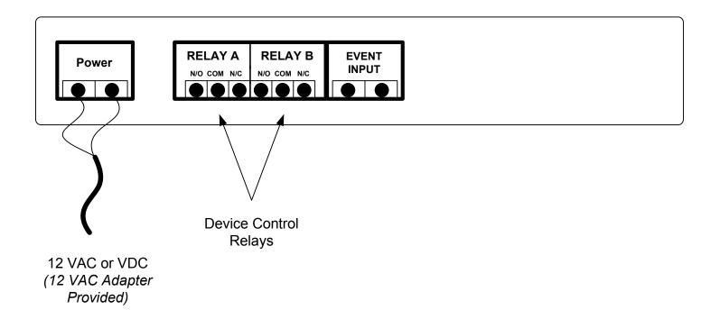
This diagram show the basic hook-ups for the remote sytation ("gatebox"). Installation is common to most keypad installations. You need two wires for power and two wires for device ("gate") control. Power is 12 volts AC or DC only and must be able to handle a 1.5 amp load.
