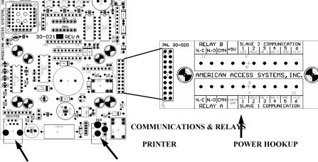
(A). Make all your prox slave connections BEFORE you apply power to the master unit. To connect power to your new desk unit plug the wall transformer into an outlet and insert the other end in the back of the unit.
