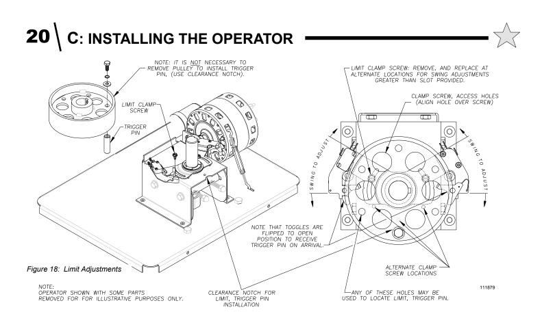
mounting hole is positioned directly above the clearance notch provided in the shaft support tower (see Figure 18). This notch provides the appropriate clearance to install the limit trigger pin with the bolt and washers provided. Install the trigger pin firmly in place.
