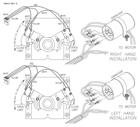
Figure 13: Left/Right Hand Installation Limit & Motor Wiring Diagram
