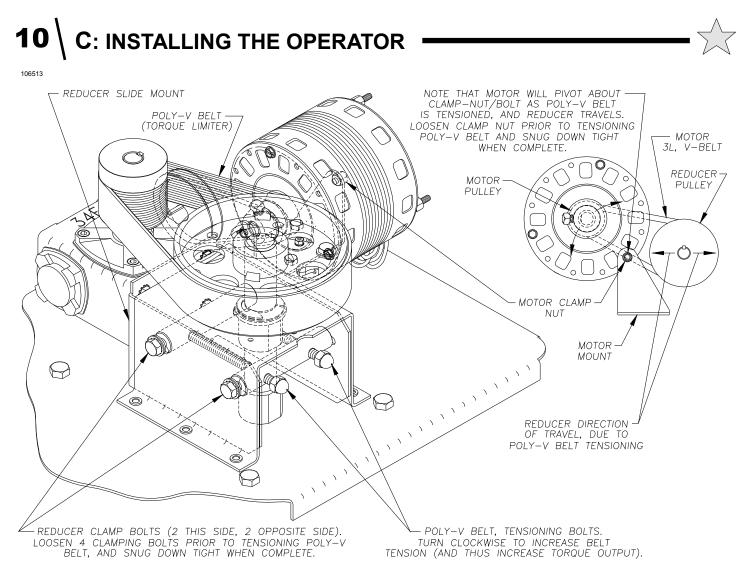
Figure 9: Torque Adjustment
