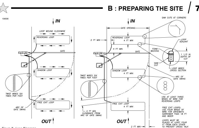
Figure 7: Loop Diagrams
