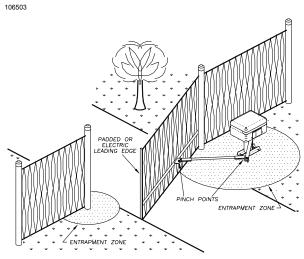
Figure 3: Entrapment Zones and Pinch Points
