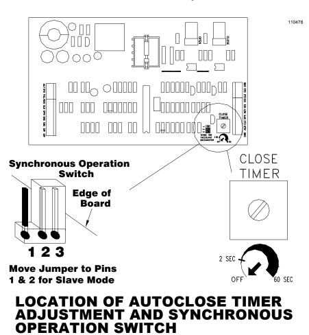
Figure 19: Timer Adjustment and Synchronous Switch Location
